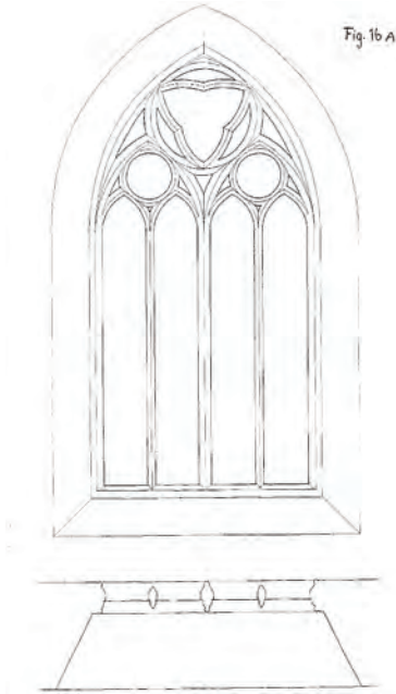
Fig. 33. Reconstruction of one of the stone tracery windows of St Mary's based on fragments found in the ruin by Randi Horgen and Håkon Christie. (After Horgen 1995: Fig. 16 A).
